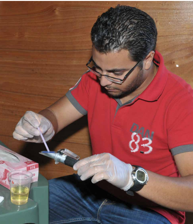
A DAN Europe researcher performs a Urinary Density test during a DAN Research event. This test determines the specific gravity of urine, which depends on the state of hydration of the diver.
